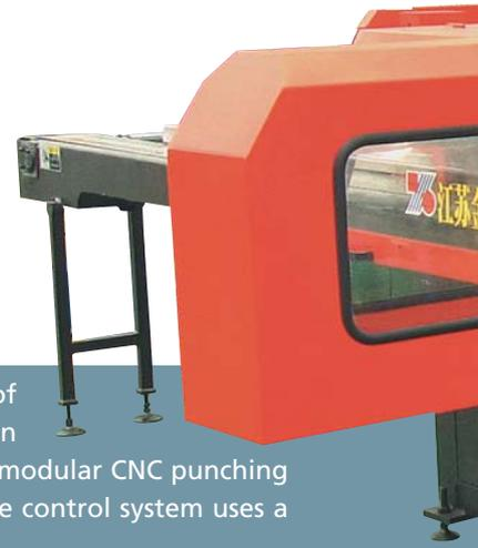
The company Jiangsu Jinfangyuan CNC Machine Co. Ltd., which is located in the high-tech area of Yangzhou City, China, manufactures and exports a wide range of hydraulic or servomotor-driven CNC machines for punching, bending and cutting sheet metal. Jiangsu Jinfangyuan developed a modular CNC punching and bending machine for producing busbars that can be operated individually or in tandem. The control system uses a PC-based automation solution from Beckhoff Automation.
