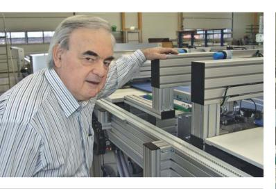
Pierre Bartholdi, Jentschmann AG: "The precise cloth length is an important quality criterion for our machines. We cut with an accuracy of  $\pm 1$  to 2 mm. The width of the cloth is regulated via an edge controller."
