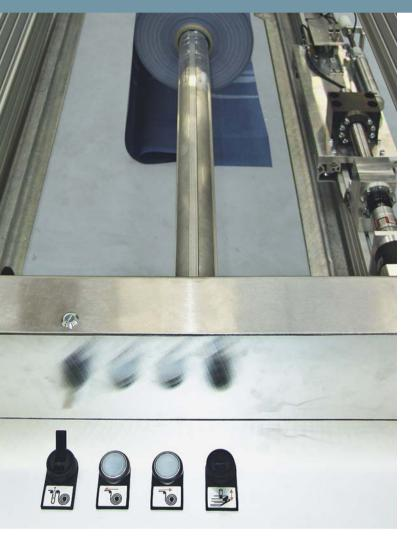
Manual control level of the web roller carriage, with which the cloth roll is driven into the machine
