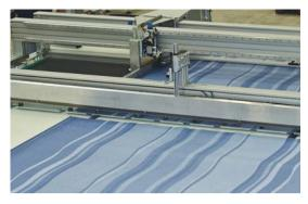
The severed awning web is removed and set down by the pulling carriage; the awning cloth is tensioned by the cutting gantry and transported further.
