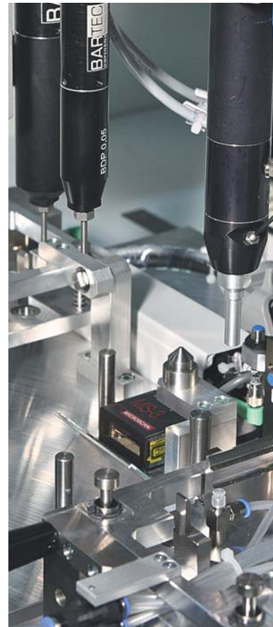
Plasma pre-treatment and double single component dispensing with a screw pump for casting electrical devices.
