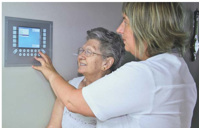
Each room is equipped with a Beckhoff Panel PC with a touchscreen. Via an identification button the caregiver can log in to enter or view data.
