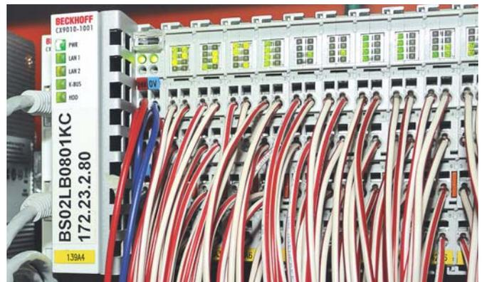
via Ethernet interfaces. A total of 655 digital inputs, 248 digital outputs, 195 analog inputs and 163 analog outputs were used. The CX9010 Embedded PCs employed, with Windows CE as the operating system, communicate all data via the TwinCAT ADS protocol.
