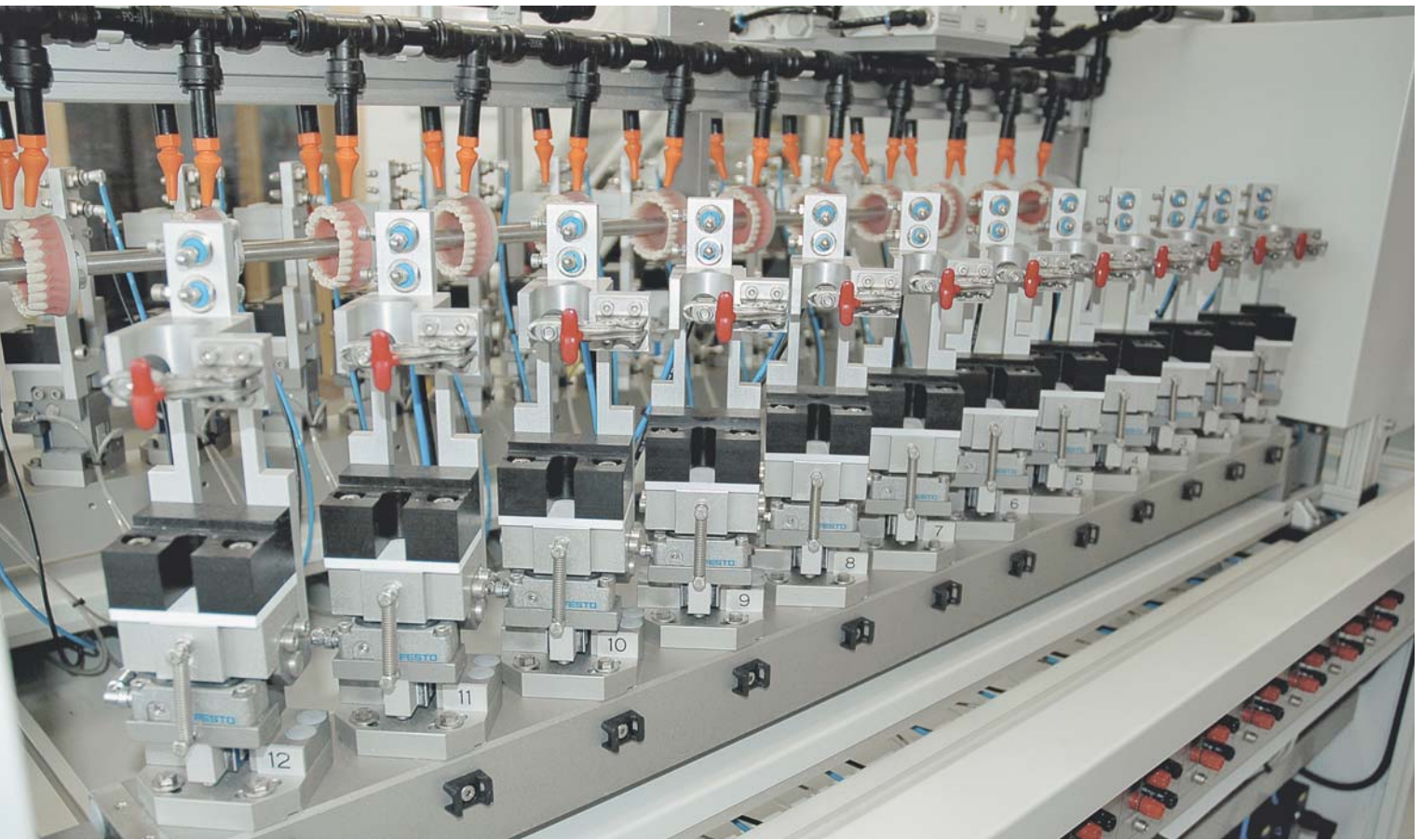
Toothbrush designs are tested according to their expected lifecycle over approx. 100 hours using artificial sets of teeth and toothpaste emulsion.
