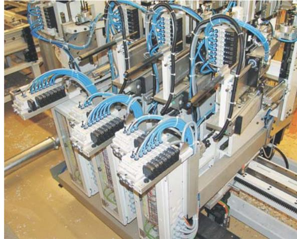
Complex structure of pneumatic valve terminals with connection to Beckhoff Bus Terminals
