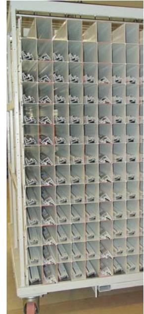
Compartment trolley for the accommodation of up to 208 machined profile sections
