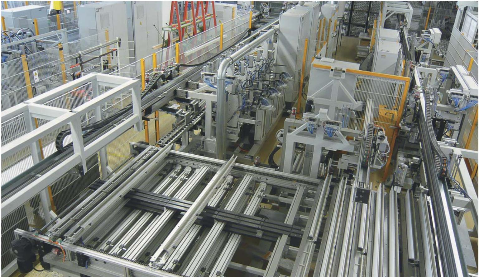
SBZ II bar processing center with insertion unit for PVC profiles up to 3,750 mm long and gripper tongs positioned by NC for positioning speeds of up to 180 m/min
