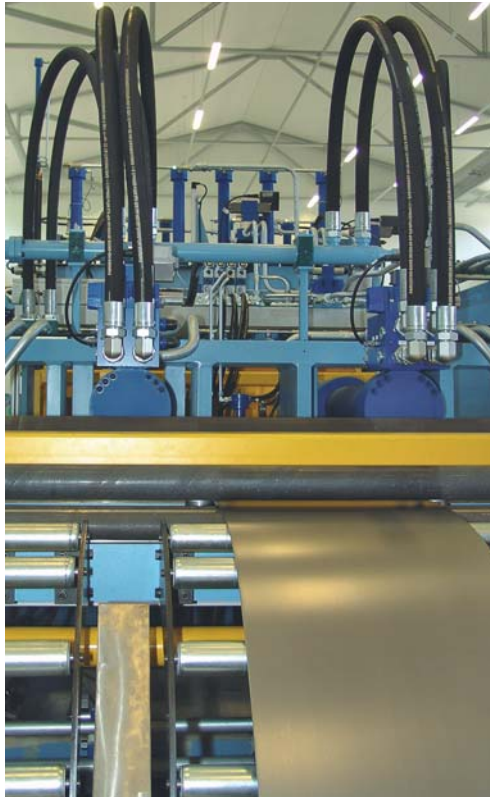
A total of 12 hydraulic servo axes produce two x 250 t hydraulic thrust in order to fold the cooling fins.
