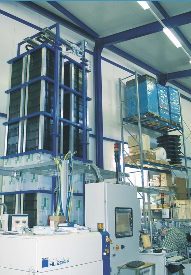
The new Pollmann production facility during the test phase at the Karlstein factory: in the foreground, the laser welding machine by Trumpf, in the background, the 4 meter high storage tower that serves for the curing of the cast parts coming from the two-component casting station. At the same time, it is used as a buffer store within the overall production process.
