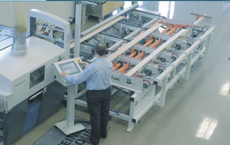
The ValuRip Plus™ incorporates a Beckhoff CP6901 Control Panel with DVI/USB interface as the HMI hardware.
