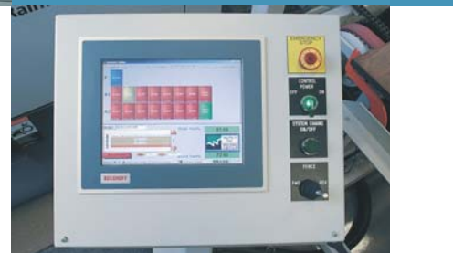
The ValuRip Plus™ incorporates a Beckhoff CP6901 Control Panel with DVI/USB interface as the HMI hardware.
