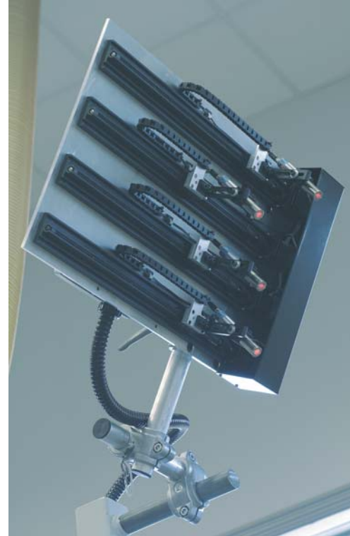
Integrated Laser Alignment Rack, controlled by a CX1020 Embedded PC
