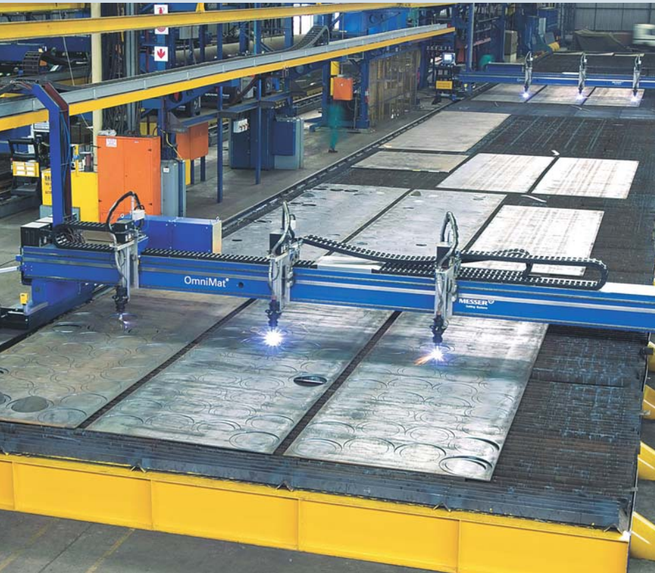
By using three HPR260 plasma cutters simultaneously, Trident Steel achieves high quality and outstanding productivity.
