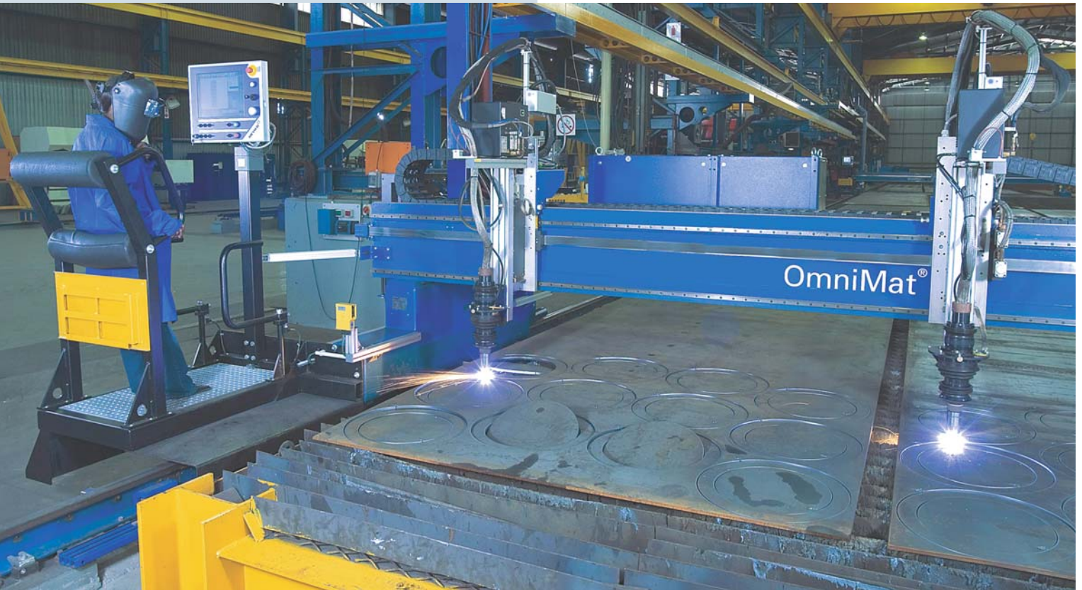
Precise, rapid cuts proceed fully automatically thanks to Messer's 'Global Control'.
