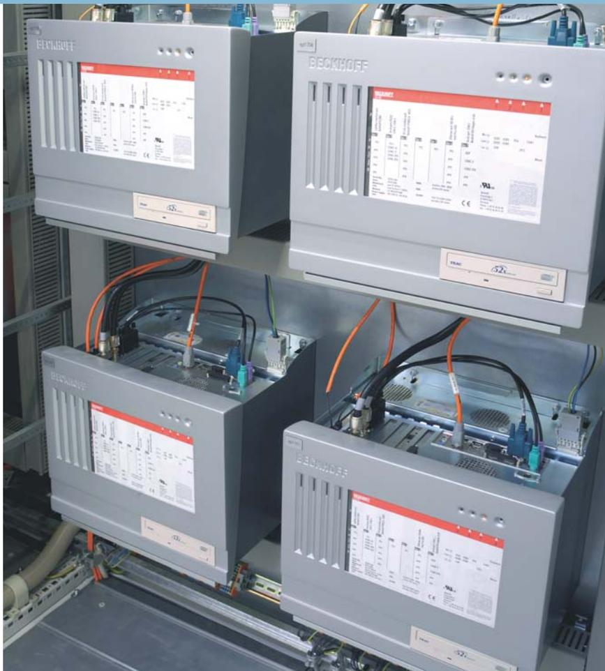
The C6140 control cabinet IPCs with CP7032 Control Panels are used for controlling highly complex drilling processes as well as for time registration.
