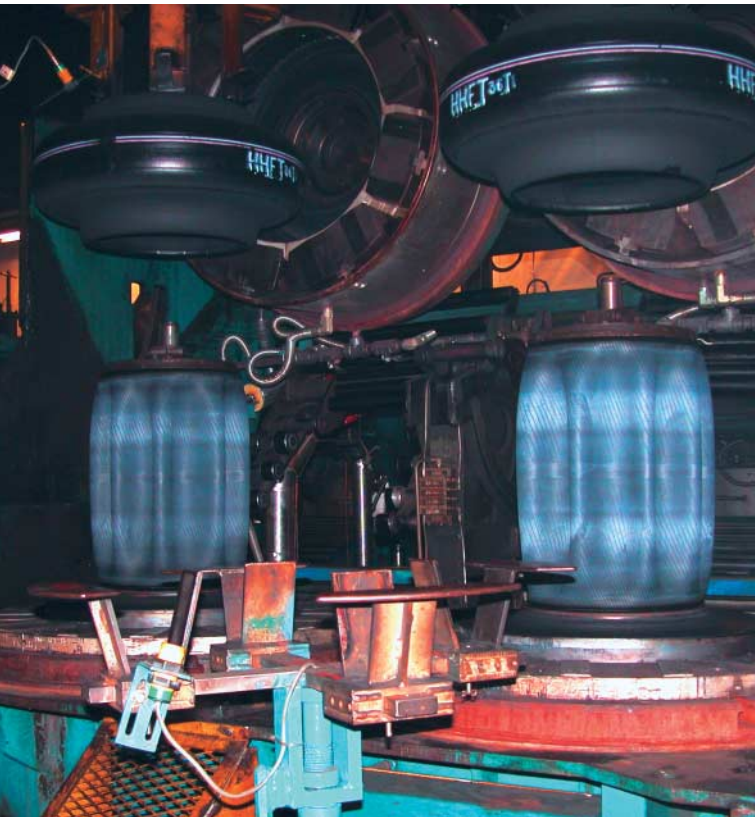
Bladders inflate inside green tires to achieve the proper shape and seam.
