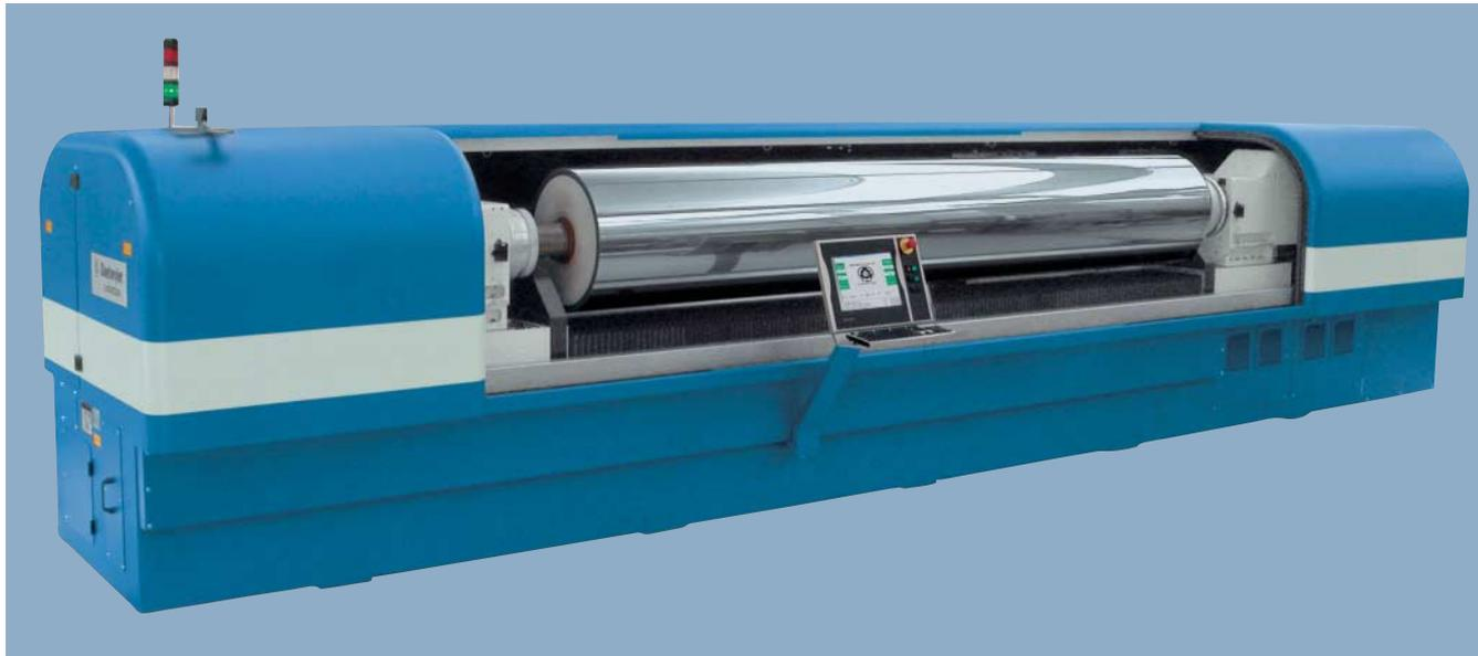
With an engraving speed of up to 35,000, optionally up to 70,000 cells per second, six NC axes, approximately 200 I/Os and two 400 W lasers, the "Laserstar" engraver is very demanding when it comes to automation engineering.
