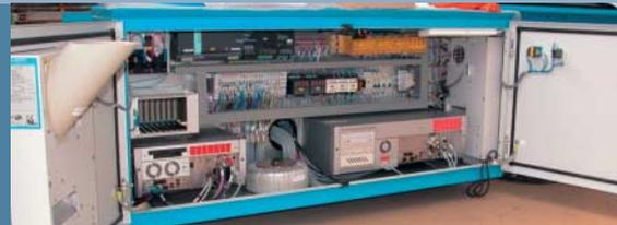
The "control center" of the Laserstar engraving machine, equipped with Beckhoff components: C6240 Industrial PC for control tasks and C6250 for visualization, PROFIBUS Bus Couplers and Bus Terminals.
