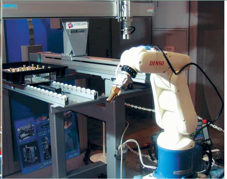
Kanto Seiki Co. Ltd. developed the Ethernet-based robot control system with BK9000 for robots with 4 to 6 axes.
