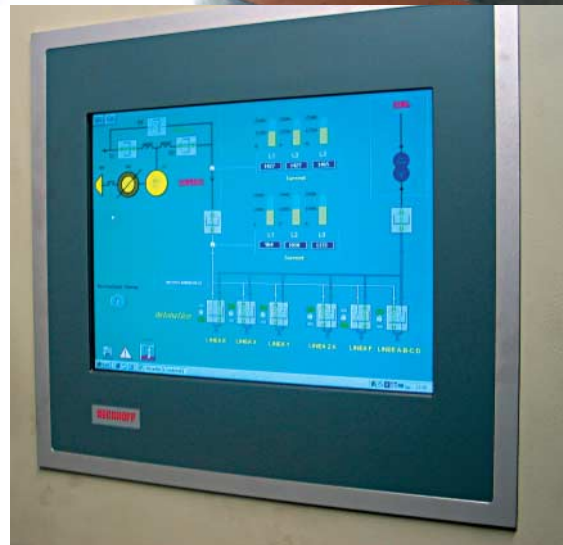
The starting point for the machine revision was the elimination of excessively long cables with the aid of 1.5 Mbaud PROFIBUS technology. The control system consists of C6130 and CP6502 (picture ahead) Industrial PCs and CP7010 Control Panels, all from Beckhoff.
