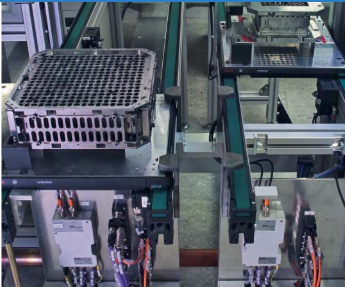
Overview of the plant: Both welding chambers are equipped with a welding laser, a camera system and a visualization PC at the control unit. A Kuka robot handles the steel grids.
