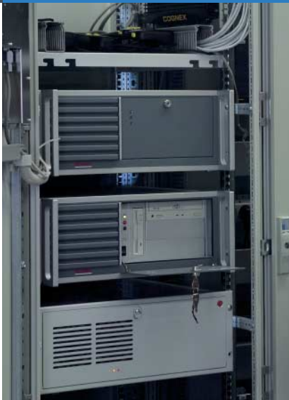
The 19-inch slide-in PC from Beckhoff serves as control PC on which the TwinCAT NC I automation software runs.
