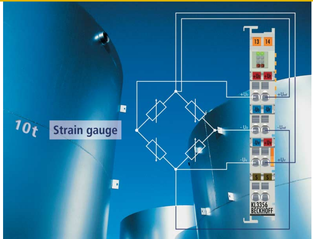
Application example: The contents of a 10-tonne silo are weighed via strain gauges and analyzed via the high-precision KL3356 resistance bridge Bus Terminal. With a minimum measurement error of <\pm 0.01\% , the total measurement error is <\pm 1\text{ kg} .
