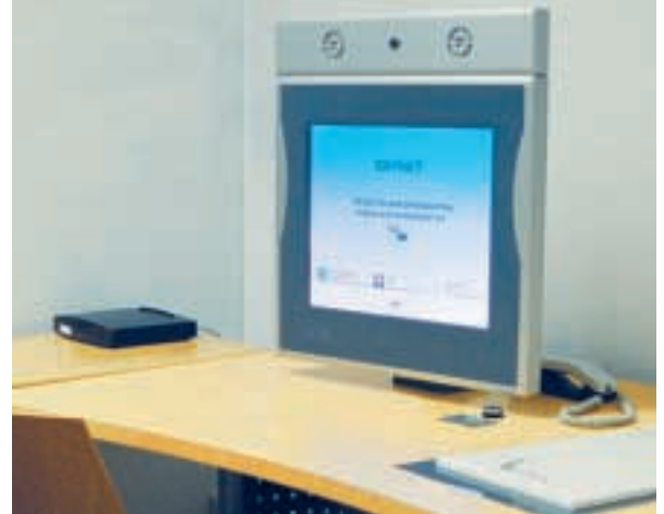
Customer-specific Control Panel from Beckhoff as a robust operating unit for the Skynet system.
