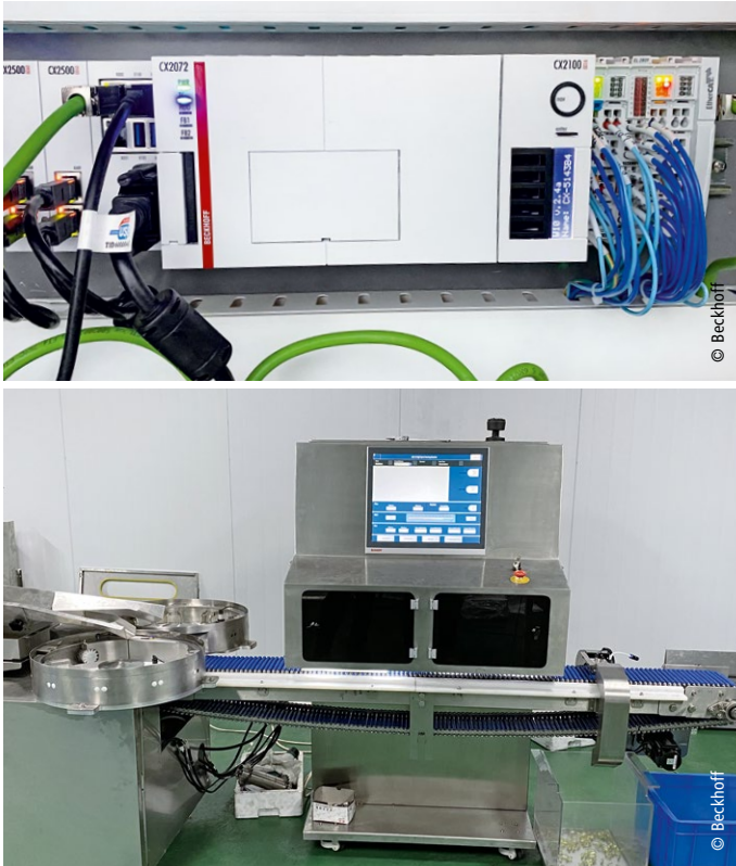
Above: A powerful CX2072 Embedded PC is used as the all-in-one control platform for the high-speed soft capsule inspection machine developed by Xin Hang Cheng.
