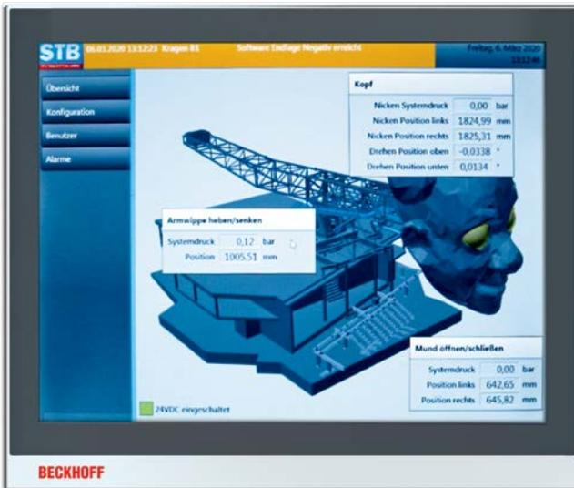
The main cabinet and the panel for controlling the hydraulics are each equipped with a built-in 15-inch CP6602 Panel PC from Beckhoff.
