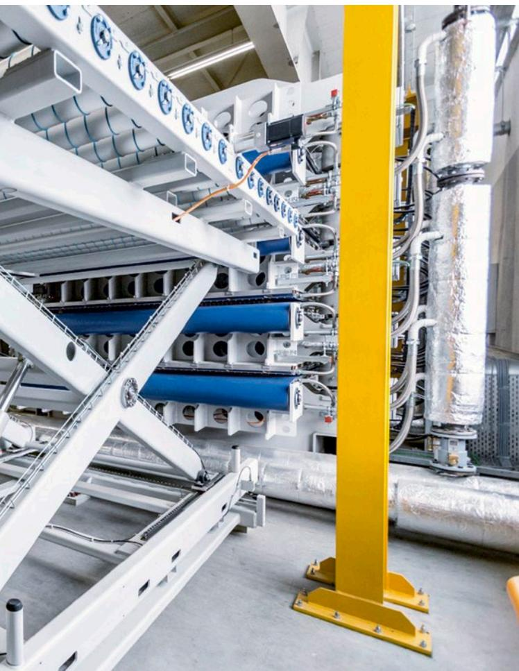
Scissor-type lifting table in the process of removing a finished Lisocore® panel from the multi-level press.
