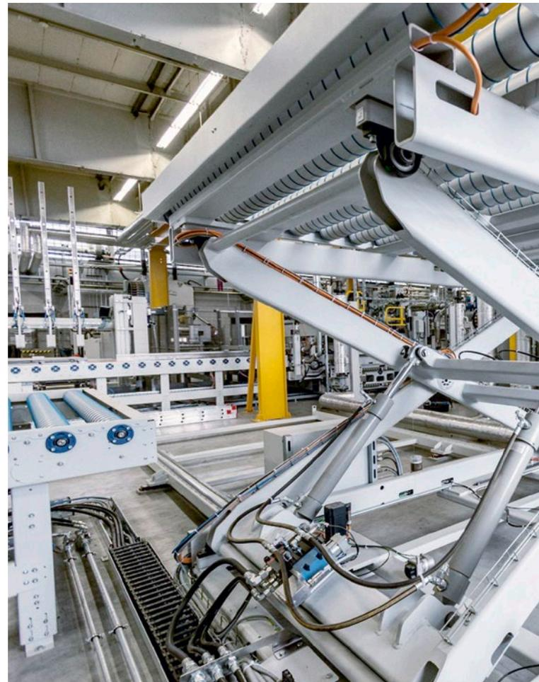
Once the protective layers and the core structure have been joined correctly, the "sandwich material", which is still quite fragile, is transferred to a hydraulically operated, scissor-type lifting table. This table transfers the incoming products to a multi-level press, where the individual elements are joined in a dimensionally accurate, permanent manner with a hardening adhesive.
