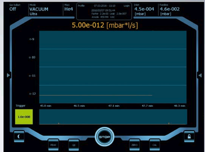
The clearly laid-out user interface of the leak detector was realized using TwinCAT 3 PLC HMI software.
