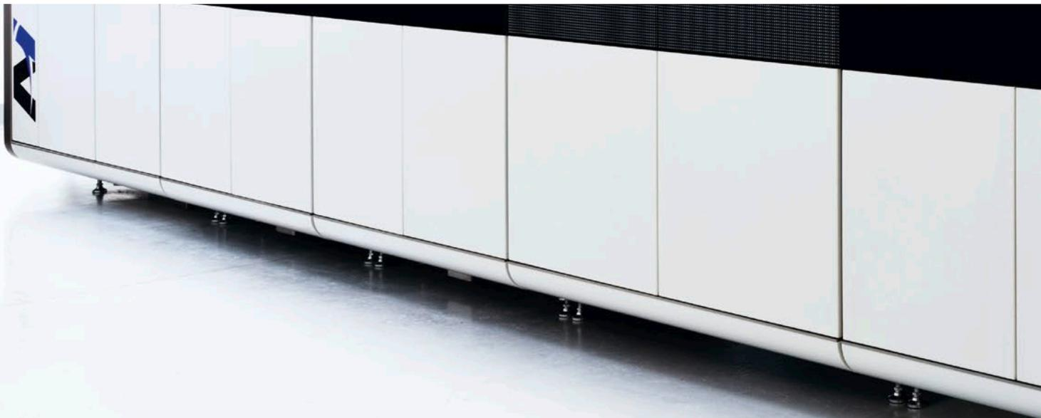
The MetalFAB1 from Additive Industries is a 3D printer for high-end applications. This system can be equipped with up to four printer modules, with different optional modules for further processing of the workpieces.
