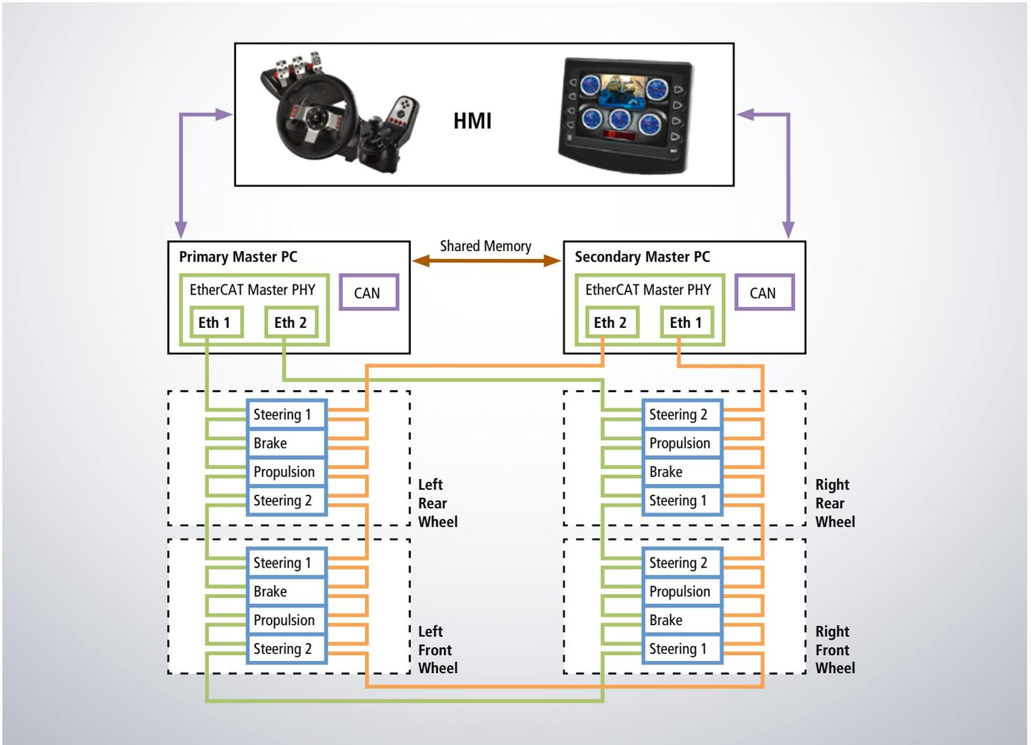
Figure 2: The controls of the MRV for each wheel’s propulsion, braking, and steering are controlled through a triple-redundant EtherCAT network.
