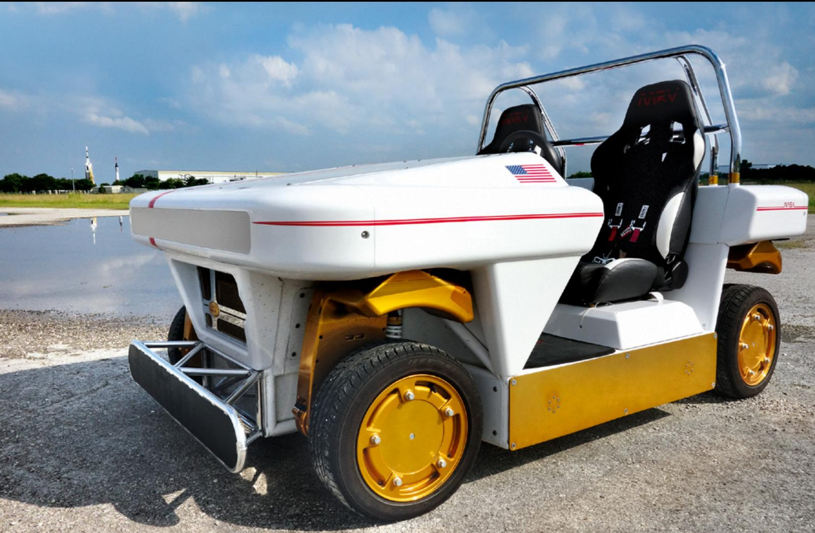
The Modular Robot Vehicle developed by NASA looks like a “roadster” at first glance, but can be more accurately defined as a robot. Having individual control of each steering and drive unit enables the MRV to travel in some very unorthodox modes.
