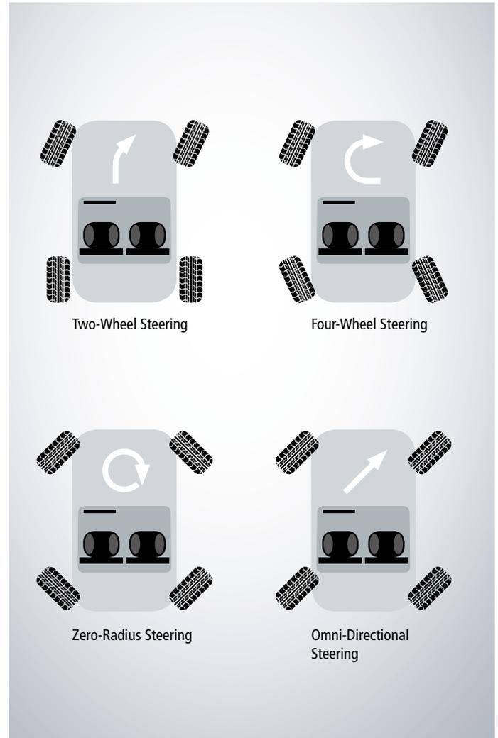
Figure 1: The MRV can drive in traditional modes, such as “two-wheel steering” and “four-wheel steering”, but it can also be switched to “omnidirectional mode”.
