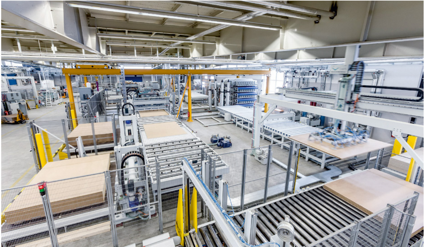
The rectilinear arrangement of the processing stations results in a highly compact and powerful machine installation.
