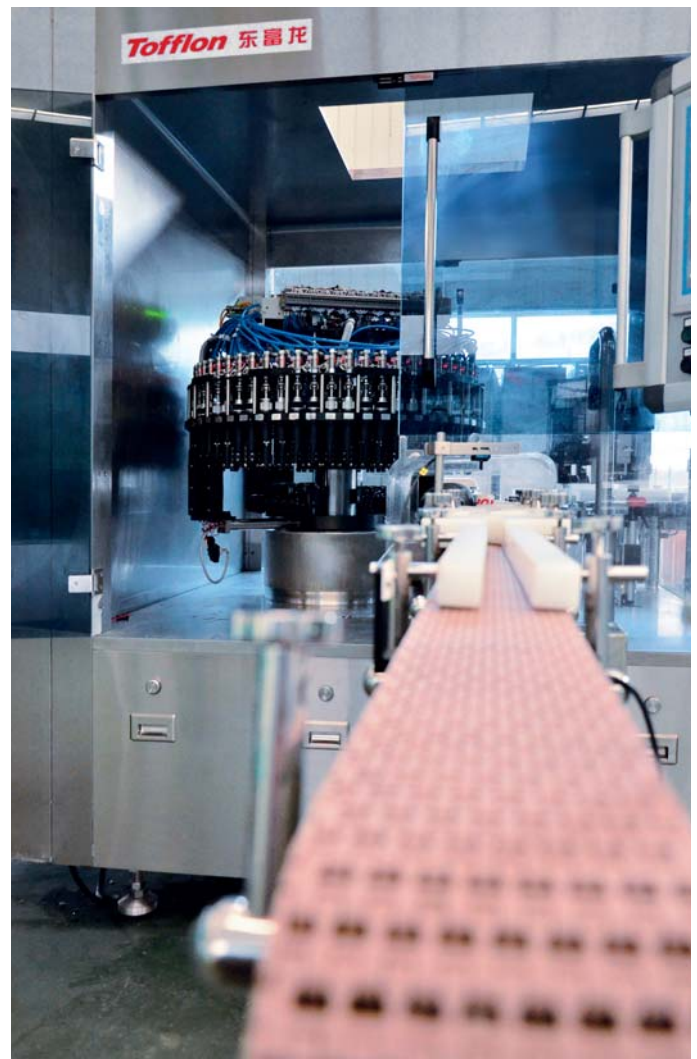
Machine for the fully automatic optical inspection of containers for freeze-dried pharmaceuticals.
