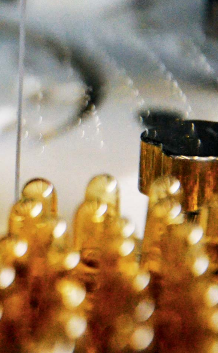
The inspection machine detects contaminants, cracks, or inclusions (microscopic imperfections) with a high degree of reliability. Faulty containers are automatically removed.
