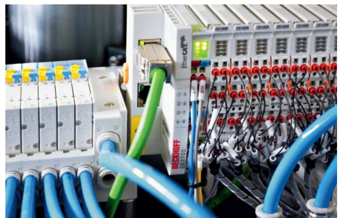
Tofflon uses EtherCAT as the fieldbus system for its inspection machine. The data is transmitted via EtherCAT Terminals and Bus Terminals.
