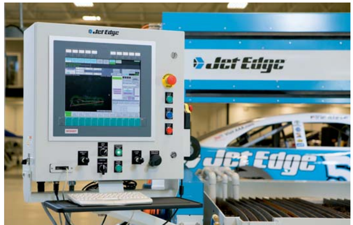
For the machine display Jet Edge uses a CP6912 Control Panel with DVI/USB extension, which can be installed up to 50 m away from the C6920 Industrial PC.
