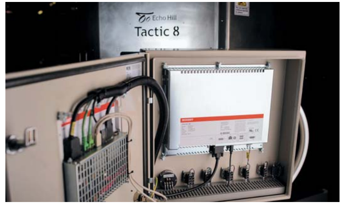
Echo Hill controls the whole grinding cell, including three robots and the measuring system, via a C6515 Industrial PC and TwinCAT automation software.
