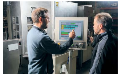
A remote "Economy" Control Panel from the CP690x series is used for machine visualization.
