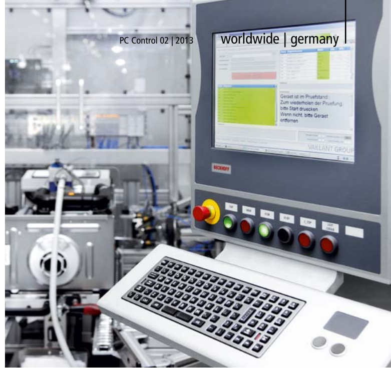
The test process can be monitored via the Beckhoff Control Panel specially customized for the Vaillant Group.
