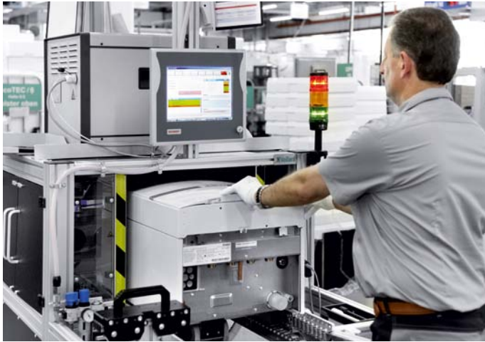
A Vaillant heating appliance is pushed into the test bench.
