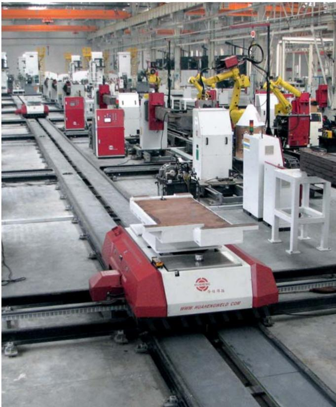
The fully automated production line essentially consists of five elements: the rail, the rail-guided vehicle as the means of transport, a robot station, a decentralized control system and the higher level controller.
