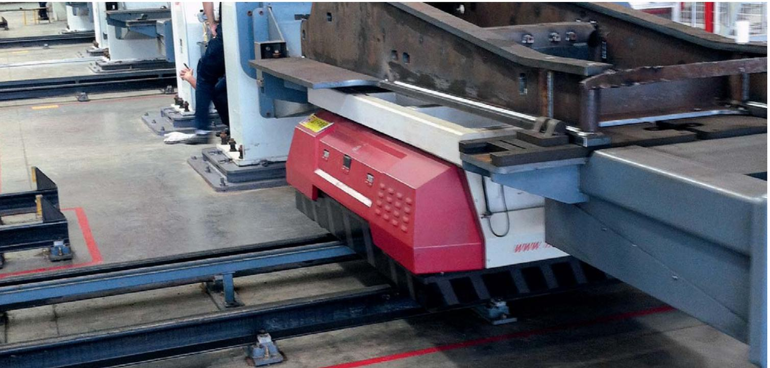
The rail-guided vehicles are used among other things for the automatic production of excavator shovels and booms in the structural welding shop at the Sany Lingang Factory, a manufacturer of construction vehicles and machines.
