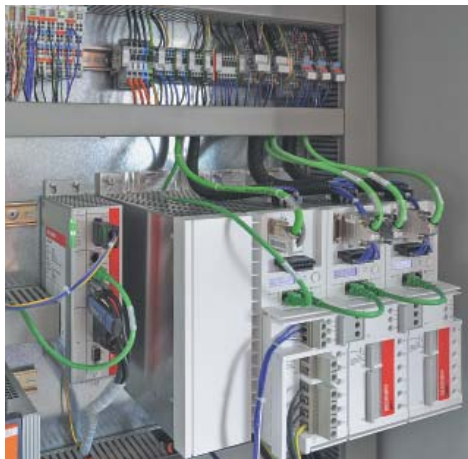
The control platform of the eCAB WorkCenter consists of a Beckhoff C6920 Industrial PC with TwinCAT NC I software, the BK1120 EtherCAT Bus Coupler and three Servo Drives from the AX5100 series.
