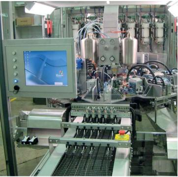
Discharge conveyor and ink processing drive platform
