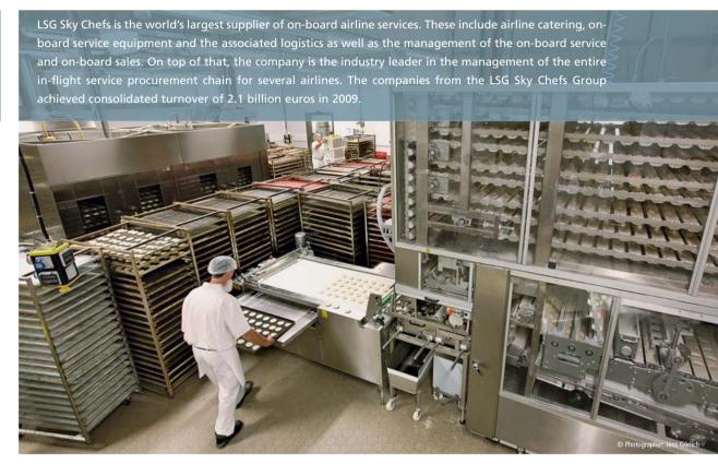
Every hour, 15,000 crusty bread rolls are produced, packed and sealed for flight in the industrial bakery in Frankfurt.
