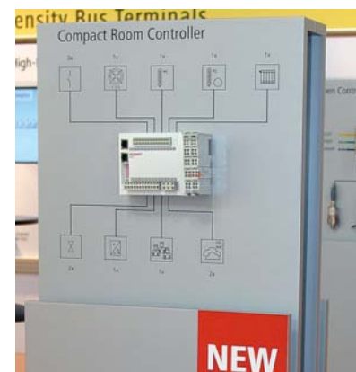
The Beckhoff BC9191 Room Controller with integrated control functionality represents a compact, low-priced solution for single room control that makes Ethernet available in each room.
