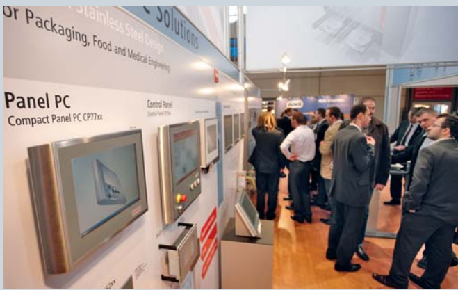
The stainless steel panels in IP 65 protection meet strict hygiene regulations.
