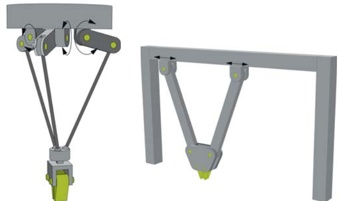
Examples of parallel kinematics: Delta and shear kinematics
