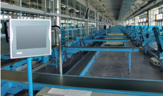
A total of 38 ramp belts are available for package loading onto HGVs. The ramp group system is controlled using a Beckhoff Control Panel.
