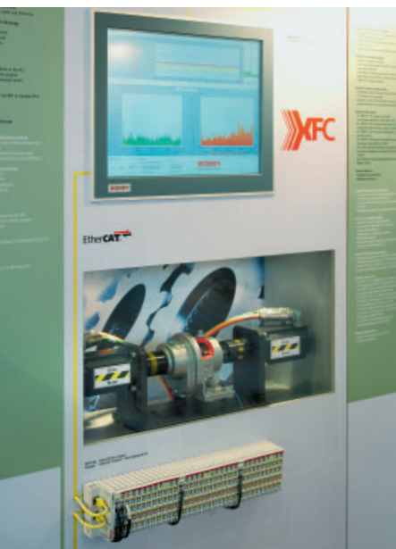
Hanover Fair 2009: Condition Monitoring solution with EL3632 EtherCAT Terminal
