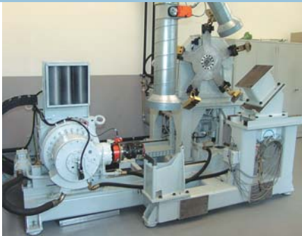
Test rig for testing the tail rotor gearbox
