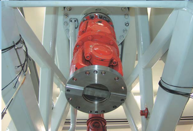
View of the coupling of electric motor drive and main rotor gearbox on the MGB test rig
