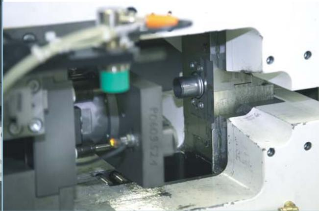
The machine has a modular structure with three main and two auxiliary stations. The parts are advanced through the machining stations by a servomotor-driven handling device. The cycle time for an assembly needing three swaging processes amounts to about 8.5 seconds per assembly.
