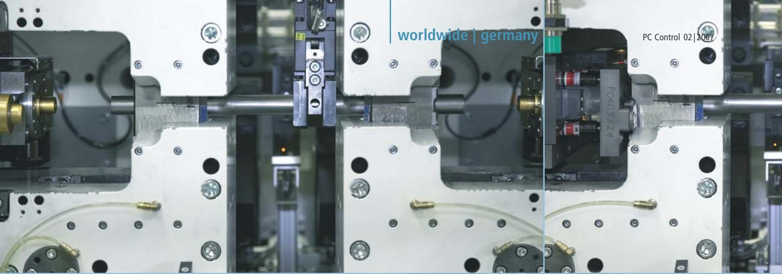
In the tube end forming machine both tube ends are hydraulically upset through cold forming. The end product is a subassembly incorporated in a unit for the motor vehicle industry.
