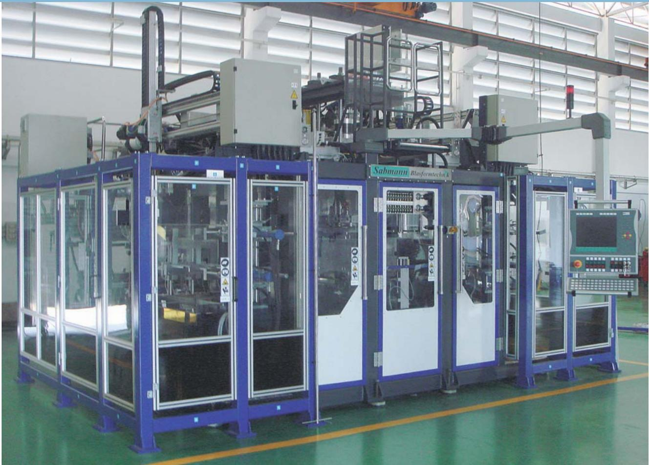
SAB is a leading manufacturer and supplier of extrusion and injection blow molding machines for the plastics industry worldwide. Previously, the machines had a special control system: Three CPUs were used for sequence programming, motion and temperature control; a different fieldbus technology was used for the controller and the I/Os. The hydraulic control system was a black box that SAB was unable to adapt or develop further.
