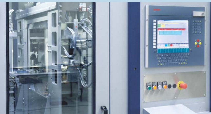
A 19-inch Panel PC C3330 with alphanumeric PC keyboard is used as PC platform for the aluminum processing center.
