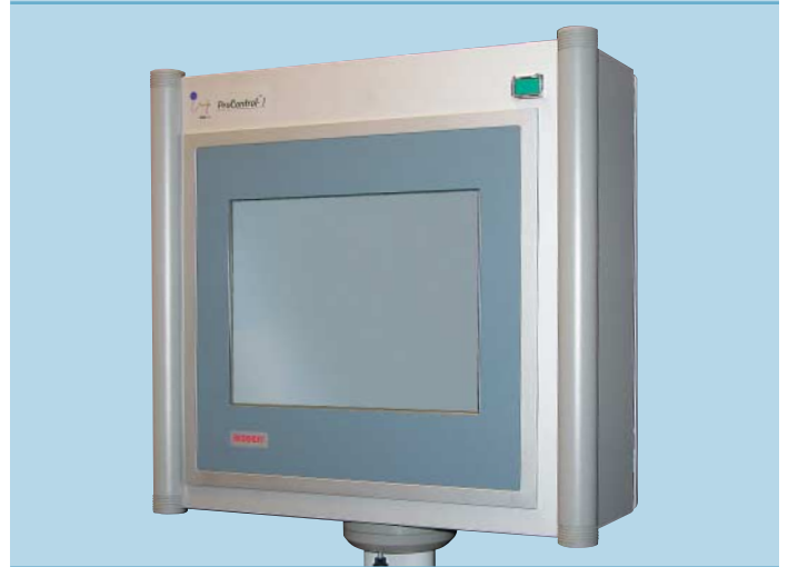
The Panel PC in the ProControl-I networks over Ethernet TCP/IP to quickly and efficiently manage promotion codes from manufacturers' databases while maintaining seamless and secure production.
