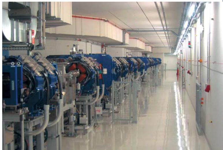
In a particle accelerator (cyclotron), protons with strong electromagnetic fields are accelerated along a spiral to 60 % of the speed of light, i.e. 180,000 km per second.
