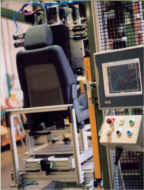
A seat undergoing sensor test and calibration in the testing station.
