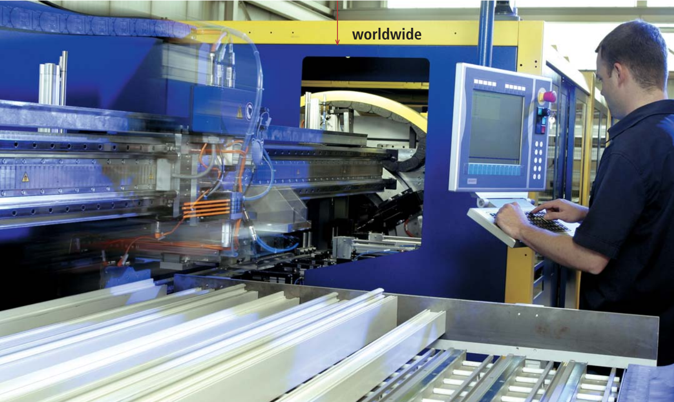
The whole system is controlled via a CP7012-1011 Control Panel from Beckhoff.
