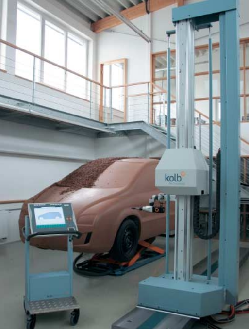
StudioLine3 CNC milling machine at the Kolb studio in Hengersberg with a 1:1 clay model and Beckhoff Control Panel on a mobile trolley.
