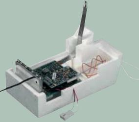
The radiosonde electronics for measuring temperature, moisture content and air pressure are protected in a polystyrene housing.
