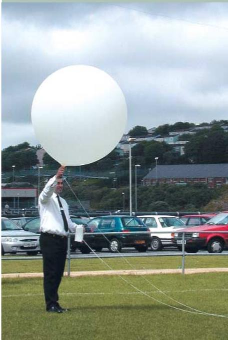
On take-off, the weather balloon with the radiosonde has a diameter of 1 to 2 m. With increasing height, the balloon becomes bigger and bigger until it finally bursts due to the decreasing air pressure.
